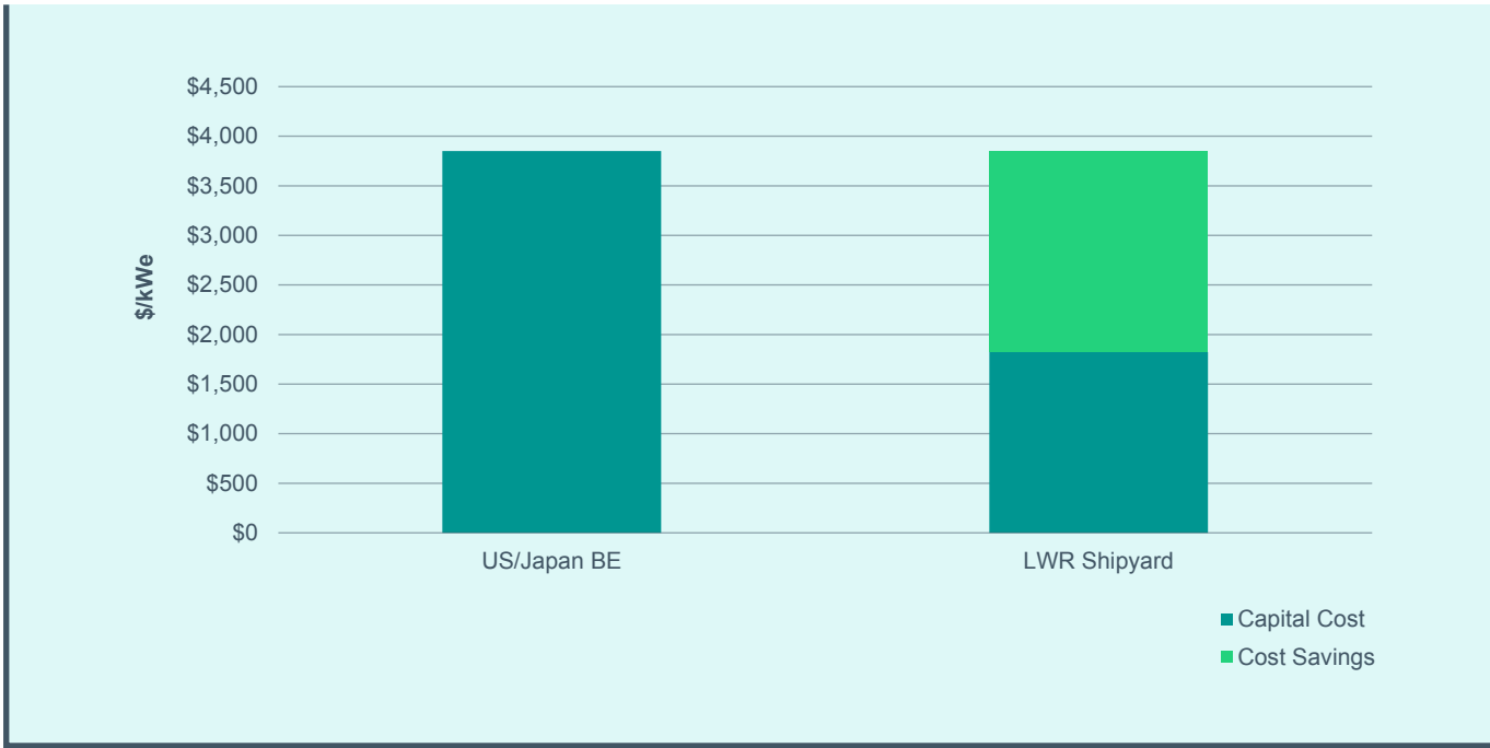
Figure 28. Costs avoided through shipyard manufacture 55
