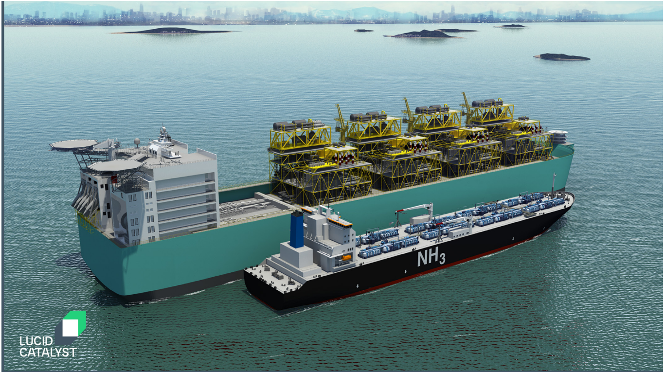
Figure 14. Rendering of ammonia bunker offloading ammonia from a production platform
